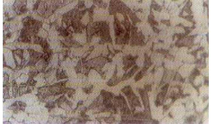
FIGURE 1 Replica of a steam drum steel subjected to overheating 200x
